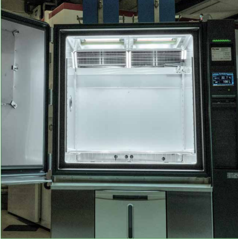
800-liter climatic test chamber with sun simulators, suitable for tests according to DIN 75220
