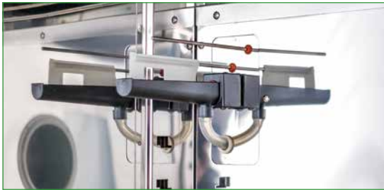
Accurate measurement and control system using a psychrometer
