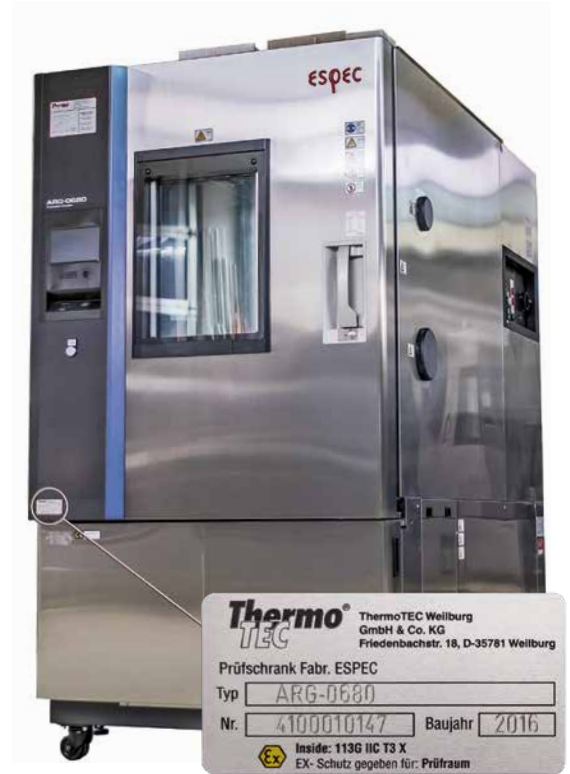
Temperature chamber according to ATEX Zone 2
