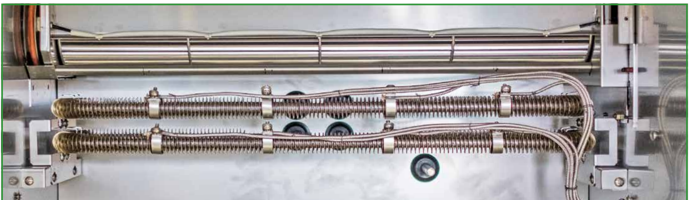
Fin heater with surface temperature measuring and limitation
