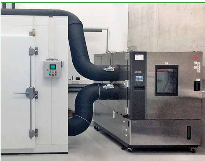
Temperature control of an external box (connected to a standard temperature chamber)
