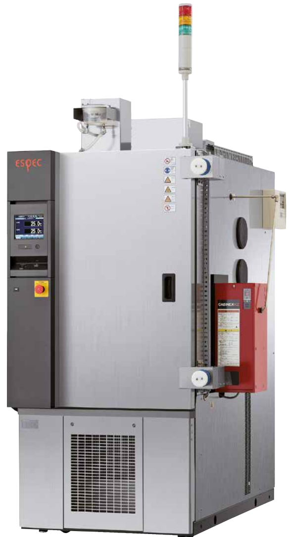
Test chamber with various safety devices for applications with batteries
